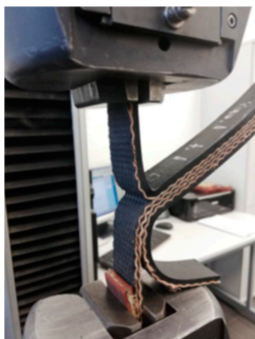
Figure 7. Delamination between ply 1 and ply 2.
